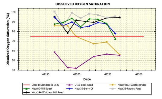
Figure 5-6-9: Graph of dissolved oxygen saturation on the tidal sites.
